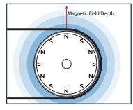
High frequency magnetic pole changes & high magnetic field strength provide superior product separation
