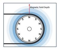
High frequency magnetic pole changes & high magnetic field strength provide superior product separation
