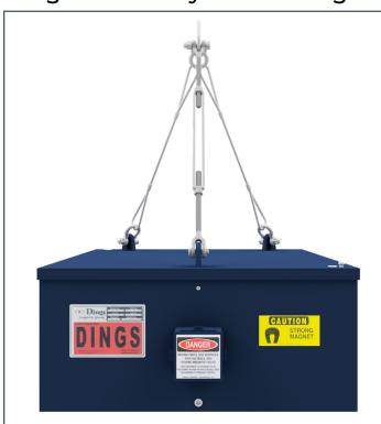
The Dings stationary electromagnet is used in applications when separation of ferrous metal is critical but not continuous. Ferrous metal collected by the stationary electromagnet is removed as necessary by cutting power to the magnet releasing the ferrous material.
