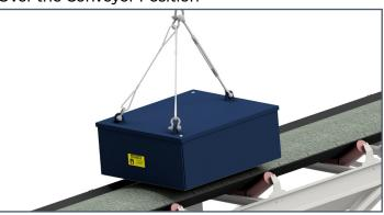
Note: Over the head pulley positioning produces the best magnet performance because the material becomes airborne, liberating the tramp metal, making it easier to separate. Inline sometimes permits use of a smaller magnet compared to crossbelt positioning. The Magnet is cleared of metal by cutting the power.
