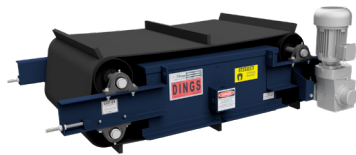
Eddy Current Separator Separate non-ferrous metal
