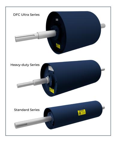
Dings Magnetic Head Pulleys are non-electric, selfcleaning magnetic separators. They operate as head pulleys on conveyors to separate tramp iron and iron impurities from materials conveyed in bulk form. They are designed for machinery protection and product purification. Our magnetic head pulley's magnetism is produced by an internal ceramic magnet assembly that is enclosed with a nonmagnetic stainless steel shell. Magnetic Head Pulleys come shipped ready to install!
