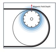
High frequency magnetic pole change & high magnetic strength provide superior product separation.
