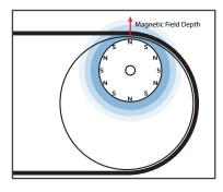
High frequency magnetic pole change & high magnetic strength provide superior product separation.
