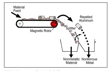
9500 Concentric Model Sizes Magnetic Pulley Diameter: 13" Belt Width: up to 72" Rotor Speed: up to 1500 rpm
