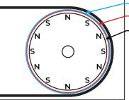
High frequency magnetic pole changes & high magnetic field strength provide superior product separation
