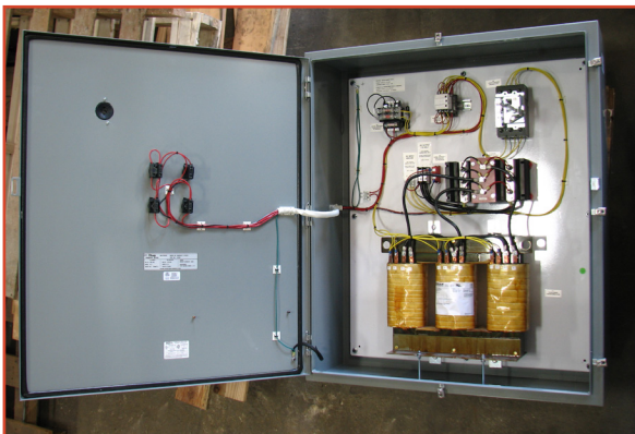
Internal Assembly of Dings Rectifier
