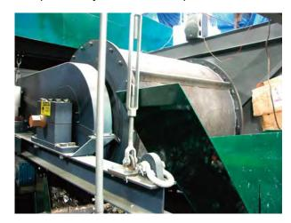
This 48" diameter x 48" width **magnetic deep draw drum** was installed to recover ferrous material. This
