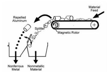
ate a magnetic field around the piece of aluminum. The polarity of that magnetic field is the same as the rotating magnet, causing the aluminum to be repelled away from the magnet.
